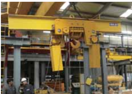
Low Head Manual Chain Hoist
