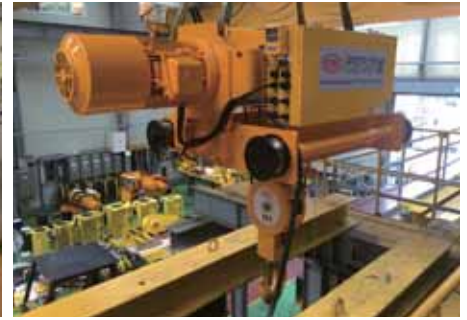
Electric Wire Hoist(10Ton)
