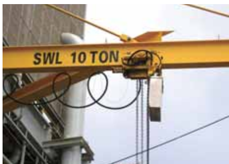
Low head type Air Hoist
